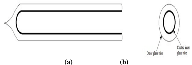
Fig. 2: Schematic diagram of evacuated tube (a) side view of evacuated tube (b) front view of evacuated tube
